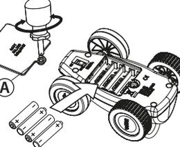
**Installing and replacing batteries:** This Action Racer is powered by 4 x AAA 1.5V batteries (not included). Use a screwdriver to open the battery cover and loosen the safety screw (A). (see illustration). Install the batteries as shown (+/-). Close the battery cover by tightening the safety screw (see illustration).
